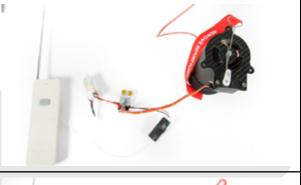
In ejection status, the angle formed has to be -45°. The pin fully release the arming rod.
